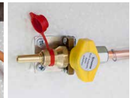
A gas outlet point in the gas storage compartment means that there is no need to pack gas bottles for the barbecue – simply hook up your grill to the caravan's gas supply.
