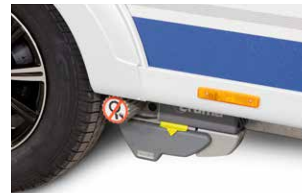
Mover automatically makes fine adjustments to the caravan's positioning, with no need for a towing vehicle.
